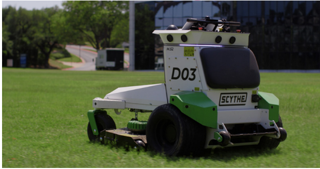
Figure 2: Scythe Sight, M.52's computer vision, uses rich visual data from the mower's eight cameras to understand the world around it (Source: Scythe Robotics)
